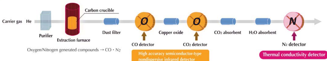
Figure 2: Gas flow diagram of the EMGA-820/EMGA-920
